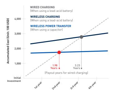
In addition to realizing reducing labor costs with complete automation using wireless charging, the manufacturer was also able to cut energy-related costs due to WPT's efficiency. By using a capacitor unit to store electrical energy in an electric field, together with the power storage device, a reduction in energy loss of only 26% was possible. Some customers achieved a yearly reduction in electricity costs and CO2 emissions of up to 60%.
